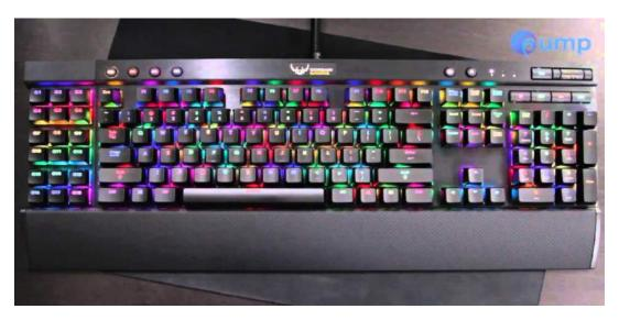
Multi-colour, per key backlighting for virtually unlimited customization every one of the keys can be assigned a unique backlighting colour. This gives you opportunities for key binding that you've never seen before in a mechanical keyboard.
