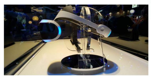
Inside the headset is a 5.7-inch OLED screen with 1920 x RGB x 1080 resolution, which comes out to about to 960 x 1080 for each eye. The PlayStation VR offers a 100-degree field of view and a 120Hz refresh rate. Latency is less than 18ms, which means that in theory it's less nausea-inducing than the previous model that had a higher latency and a slower refresh rate. There's also a jack for headphones and support for 3D audio, which will come into play later.
