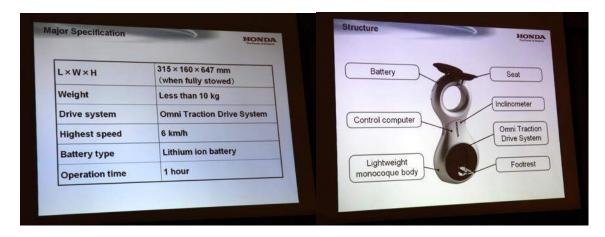
It has a top speed of 6 kilometres per hour, which is a little better than the average\_walking\_speed of an adult, and the lithium-ion battery will let us ride around for an hour. The machine weighs less than 10 kilograms (22 pounds) and max rider weight is currently100kg(220lb.).
